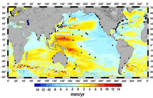
effect on regional sea level trends of the transition from ITRF2008 to ITRF2014 [Beckley et al., 2016] **Right.** Errors in vertical velocities *mm/vr)* computed with the errors in origin rates of ITRF2008 estimated by Wu et al. [2011], following Collilieux & Wöppelmann [2011].
